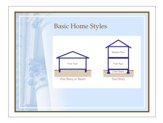
The ranch on a concrete slab reduces cost and simplifies construction.
