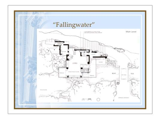
Floor plan of main level. Most of the house's floor space is devoted to the stone-paved living area with its various activity spaces. A high proportion of the living space is outdoors in the form of terraces, loggia and plunge pool below the living room.
